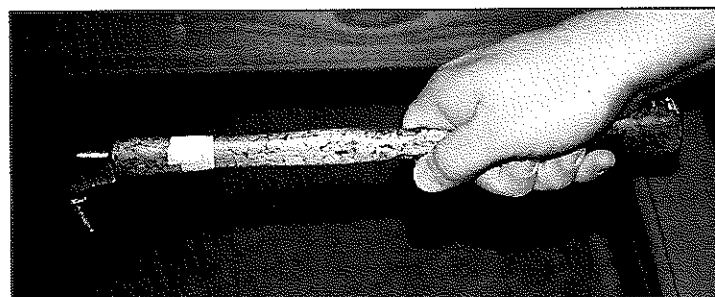
STRAIGHT WRIST. Notice straightness of wrist and position of thumb on handle. This handle for Heller 12-ounce driving hammer was cut at 13 inches and modified to fit shoer's hand.
